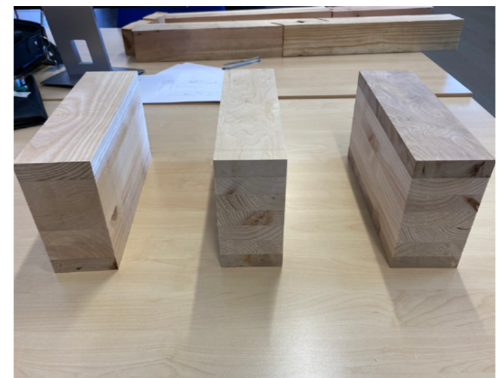
Figure 13. Hybrid glulam samples. Photo: Wojciech Plowas
