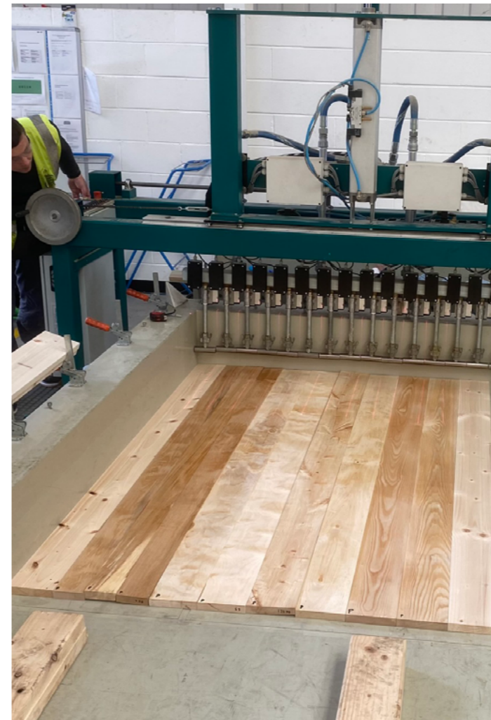
Figure 11. Hybrid CLT manufacturing. Photo: Wojciech Plowas
